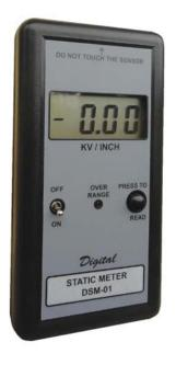
The model DSM-01 is a light weight non-contacting static meter to measure static voltages with a polarity on objects & surfaces. The unit gives direct readings of electrostatic potentials on any surface, when held at a distance of 1 inch. However, virtually higher electrostatic potential can be measured by proportionately increasing the distance from the meter to the charged object. The instrument features large display with a very low drift circuit to give measurements.
